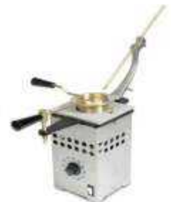
Cleveland Flash & Fire Point Apparatus
