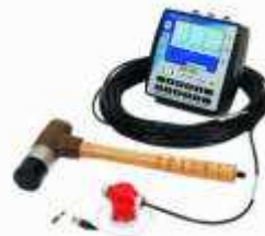
Pile Integrity Test
