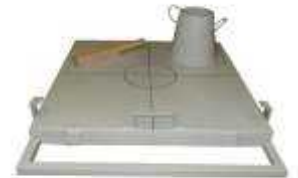
Concrete Flow Table Test Set
